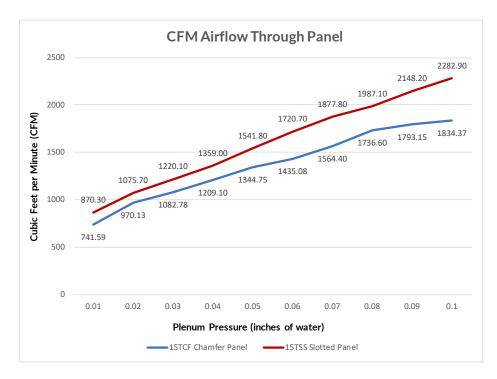
At RLE, we focus on CFM. We know the air that flows *through* the panel is more important than the open spaces cut into the top of the panel.
